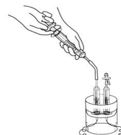
Figure 2. Filling up the “electrolysis syringe” with the sample
